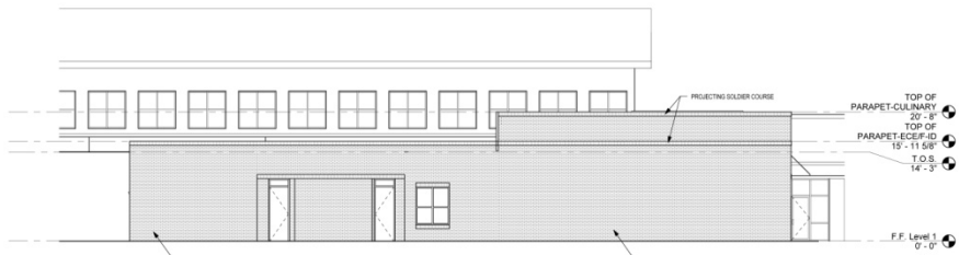
3 CULINARY - EAST ELEVATION AA.1 SCALE: 1/8" = 1'-0"
